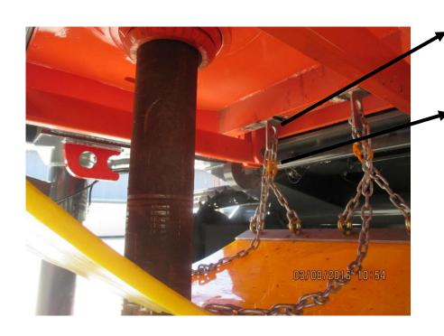
NOW ATTACH THE FRONT HANGERS BY LIFTING THE 'TAIL' OF THE CHIP MAT TO LOCATE A SOLID SUBFRAME TO WELD 2 T BRACKETS DIRECTLY ABOVE THE YELLOW HAMMER LOCKS
