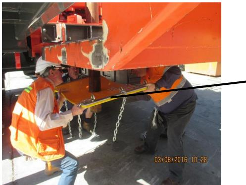
➤ USING 2 PEOPLE LIFT THE 'HEAD' OF CHIP MAT OVER THE PIPE TO MAKE A 45° ANGLE AT THE PIPE AND MARK THE FIRST 'T' BRACKET POSITION AT THE CENTRE OF THE REAR UNDERDECK
