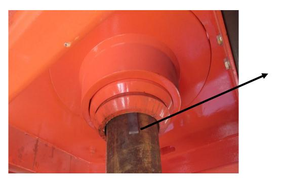
CENTRE THE DRILL PIPE WITH SHIMS
