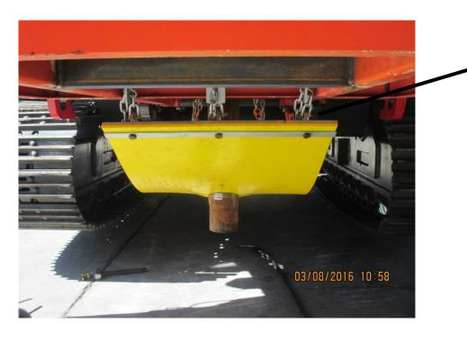
TACK WELD AND PULL CHAIN LINKS UP HIGH TO HAVE THE MAT ABOVE HORIZONTAL
