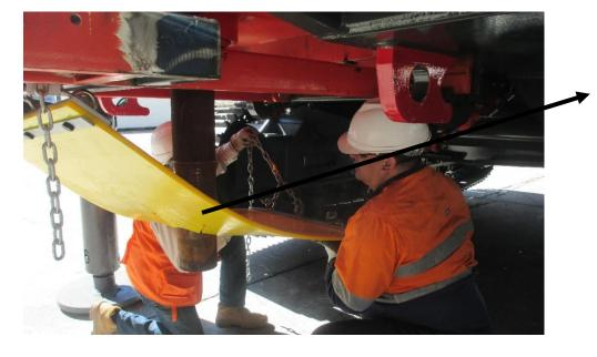
WITH AT LEAST 2 PAIRS OF HANDS LIFT THE 'HEAD' OF THE DEFLECTOR OVER THE DRILL BIT
