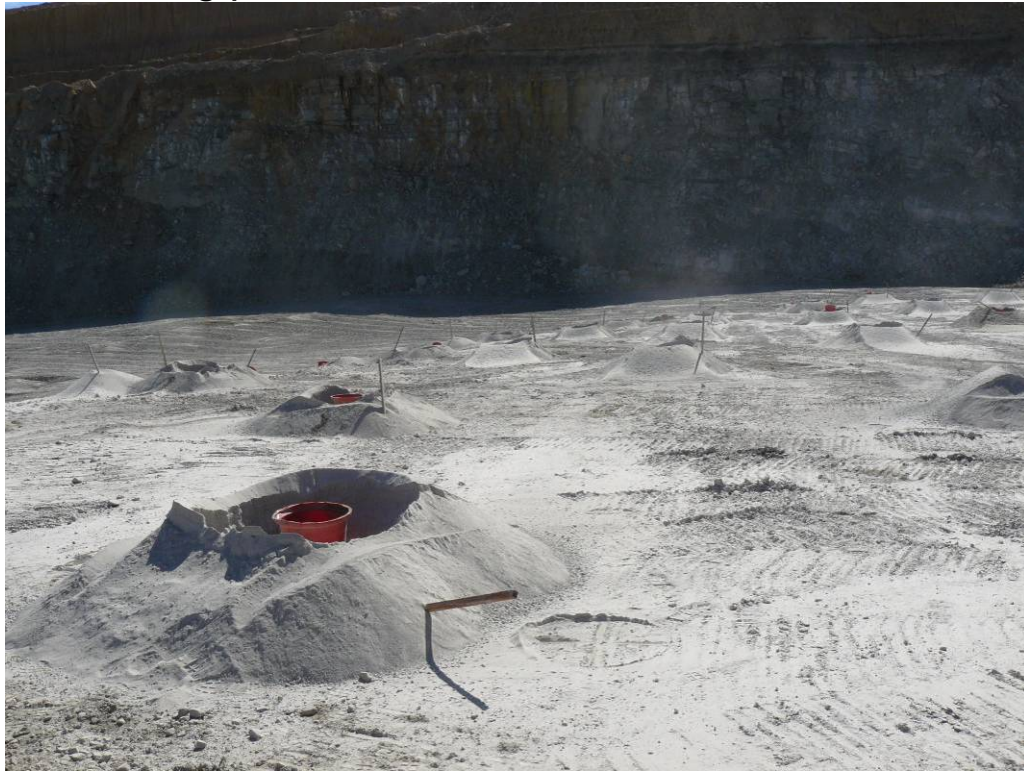
Bad cutting piles and fallback
