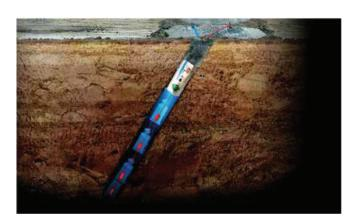
Contamination of creeks and ground water is a major concern. In holes with dynamic water, gels and emulsions can get washed out and enter the water table. Having a sealed charge eliminates the problem.
